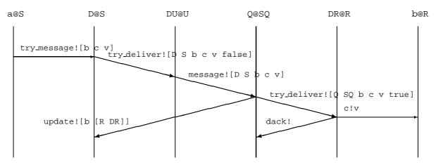
Horizontal arrows are synchronised communications within a single machine (using **iflocal**); slanted arrows are asynchronous messages.
