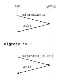
The query server's lock is kept during the migration. The agent's own record of it's current site and daemon must also be updated with the new data [U DU] when the agent's lock is released. Note that in the body of the encoding the name DU of the daemon on the target site must be available. This is achieved by encoding site names in the high-level program by pairs of a site name and the associated daemon name; there is a translation of types
