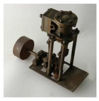
Figure 70: Steam engine with flywheel
