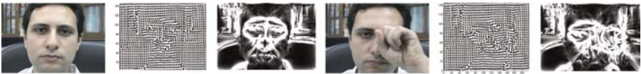
Fig. 3. (left to right) raw image, angles representing force direction, lighter areas represent discontinuities or well positions. Note the change in well positions as the hand occludes the face.
