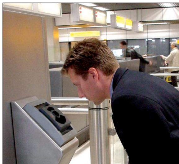
Figure 4: An infrared wavelength iris camera, using the same Daugman algorithms for iris recognition at Schiphol Airport, NL
