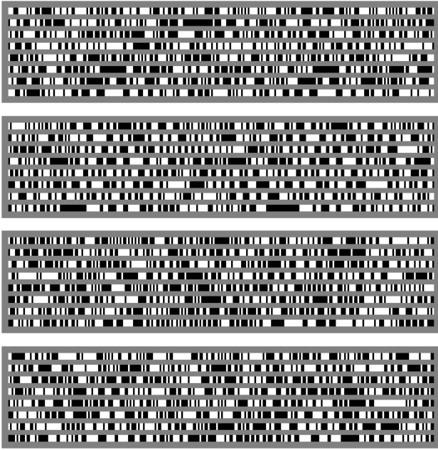
Fig. 4. Graphical portrayal of the IrisCodes produced by four different eyes. In each case, the bit streams from two different wavelets are concatenated.
