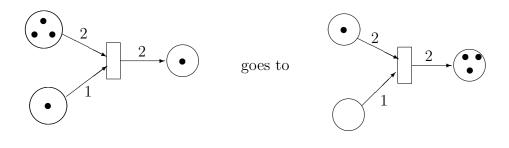
(2) The following simple net represents, for example, a buffer which can store up to five identical items, into which an item is put on each occurrence of the event in. Initially it contains three items. The event in has no preconditions so can occur provided in so doing it does not cause the capacity to be exceeded. Consequently, the event in can only occur twice.
