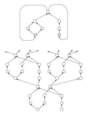
A Petri net and its occurrence-net unfolding
