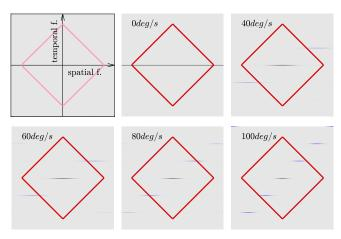
Fig. 3. Illustration of aliasing copies (blue) of the original signal (black) in the frequency domain. The spatio-temporal spectra illustrate a line moving with constant velocity (top-left corners) on a high-persistence display with a fixed refresh rate. The red diamond represents the window of visibility [Watson et al. 2008]. Higher velocities push the copies closer.
