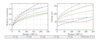
Fig. 21. Model predictions for predictable motion for different velocities (colors) in deg/s (dps) plotted against Debattista et al. [2018] (dashed line). Assuming viewing distance of 108 cm and a field of view of 30°. Resolution is relative to linear image size; Refresh rate predictions are for QHD resolution.
