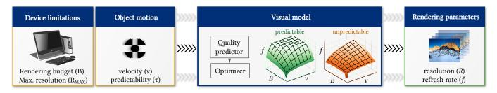
Fig. 1. Our proposed perceptual model of motion quality takes object motion, refresh rate and device limitations (such as the rendering budget and the maximum screen resolution) to predict the perceived quality. This model can be then used to find the combination of resolution and refresh rate that produces the highest animation quality under the given conditions. Surface plots visualize model predictions.
