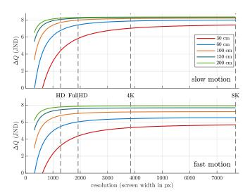
Fig. 18. Predictions for perceived quality on a 15" display with varying resolutions (horizontal axis) and viewing distances (colors). Top: slow panning motion with the content moving horizontally across the entire screen in 6.2 s; Bottom: fast motion with content moving across the entire screen in 1.5 s. Higher resolutions bring diminishing quality gains, especially when viewed from far. Closer viewing distances also result in higher angular velocities with more visible motion artifacts.
