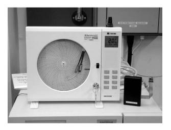
**Figure 2.18.** A paper chart temperature recorder and a PEN temperature sensor (courtesy of AT&T Laboratories Cambridge).
