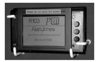
**Figure 2.19.** A dynamic room tag combining PEN, a cholesteric display and a data feed from the Active Badge system. Because they are wireless, such tags can be very easily deployed throughout a building (courtesy of AT&T Laboratories Cambridge).
