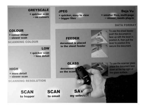
**Figure 2.13.** A smart poster acting as the computerless user interface for a public document scanner nearby. The user is about to scan the document currently on the glass (courtesy of AT&T Laboratories Cambridge).
