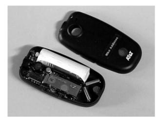
Figure 2.12. The Active Bat (courtesy of AT&T Laboratories Cambridge).
