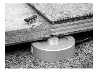
**Figure 2.11.** A detail of the construction of the Active Floor, showing a bare tile, a carpeted tile and a load cell (courtesy of AT&T Laboratories Cambridge).
