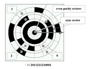
**Figure 2.14.** A TRIP target, showing (anticlockwise from East) the sync sector, the two redundancy sectors and the remaining 13 data sectors, for a total of 3<sup>13</sup> valid codes (courtesy of AT&T Laboratories Cambridge and Diego López de Ipiña).
