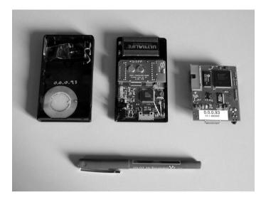
**Figure 2.16.** A PEN node, revealing its insides, and a lowercase pen for size comparison (courtesy of AT&T Laboratories Cambridge).
