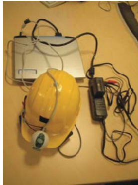
Fig. 1. Equipment required for the tetherless version of our system: a laptop, a helmet with an HMD and a camera, and the HMD electronics unit.
