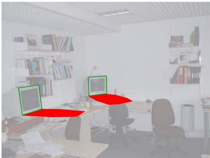
Fig. 4. Users see the teleport regions through their glasses. The regions are shown just below both monitors (The HMD is see-through, so the real-life scene is not present in the computer-generated image. Therefore, the composite must be simulated in order to show it here.).
