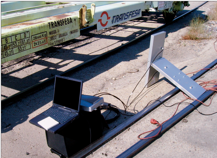
Figure 3. The test setup, showing RFID equipment for range measurements, using 2.5 cm × 2.5 cm tags on moving targets.
