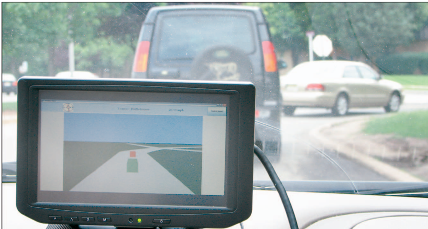
Figure 1. TrafficView's near-view panel displays cars as green or red rectangles, depending on their speed relative to the current car. In the picture, the car in front of the SUV brakes and becomes red in the panel.
