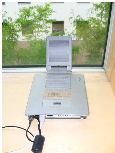
Figure 3.13: The Cisco 1200 series AP with omnidirectional patch antenna used for 802.11a experiments.
