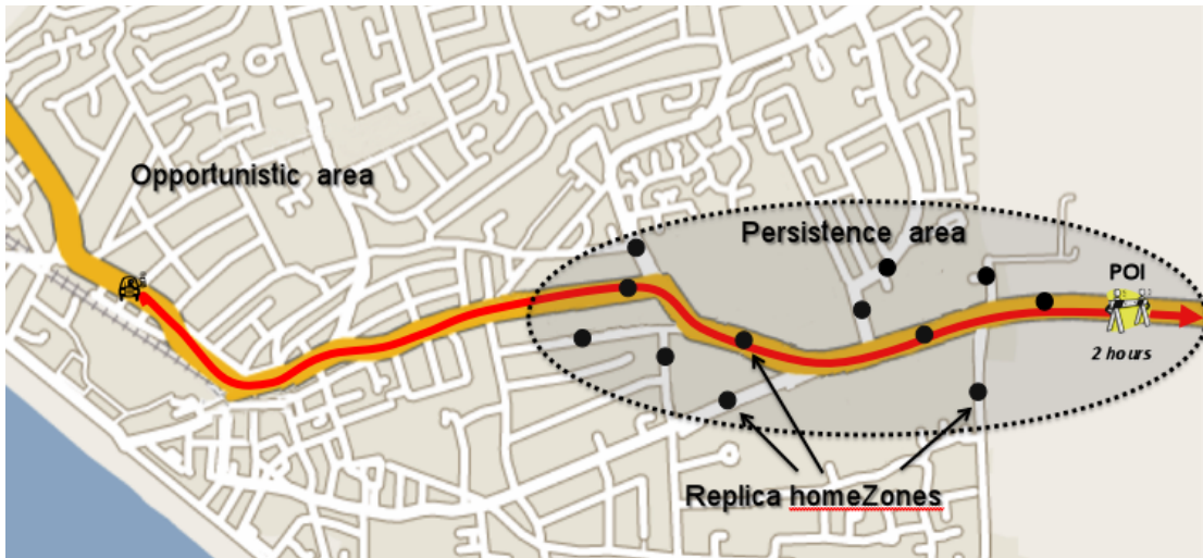
Figure 3.2: Information should be disseminated in the persistence area throughout the dissemination time. Black dots are the locations of the homeZones. In each homeZone a notification replica will be maintained. Interested vehicles driving through these locations should be notified. The information can further spread opportunistically outside the persistence area.
