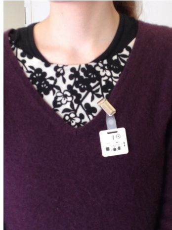
Figure 5.1: One of the RFID tags used in data collection, worn on the chest as in the deployments.
