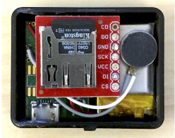
Figure 1: Electronic components enclosed in 3D printed box. The dimensions of the box are 3x4x1.5cm.
