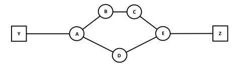
Per-packet load balancing by A and E means packets may be sent on any valid path. No firewalls or packet filtering is used anywhere in the network.
