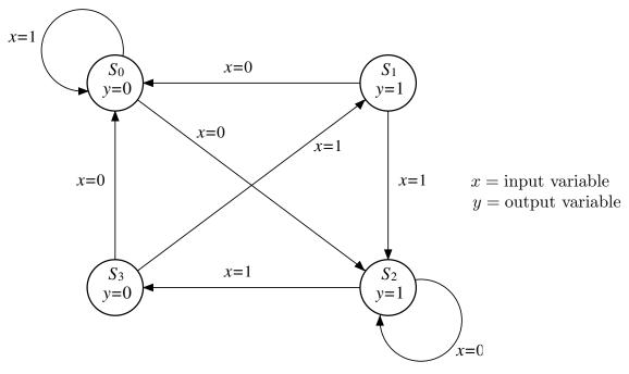
and the state assignment  $S_0 = 00$ ,  $S_1 = 01$ ,  $S_2 = 10$  and  $S_3 = 11$ .
