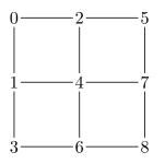
By inspection, it is clear that to get from vertex 0 to vertex 8 there are just six routes in which progress is always from a lower-numbered vertex to one with a higher number.
