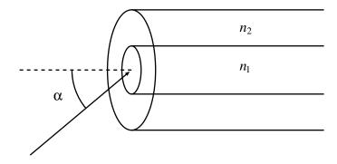
The refractive indices of the core and cladding are  $n_1$  and  $n_2$  respectively, where  $|n_1 - n_2| \ll 1$ . Prove the following condition for the incident light to be guided by the fibre
