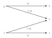
The binary erasure channel (shown above) takes as input symbols '0' and '1' and outputs '0', '1', and '?' with the probability of correct reception of a symbol being p and of erasure 1 - p. What is the capacity of this channel? [8 marks]
