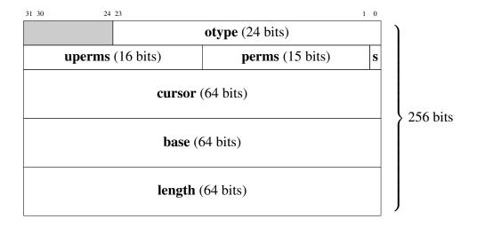
Figure 5.2: 256-bit memory representation of a capability
