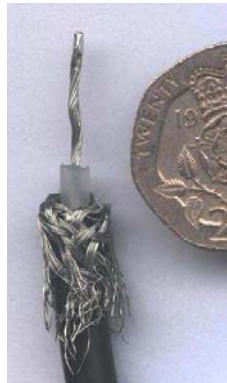
Figure 4.1: Electric field dipole formed from stripped coaxial cable
