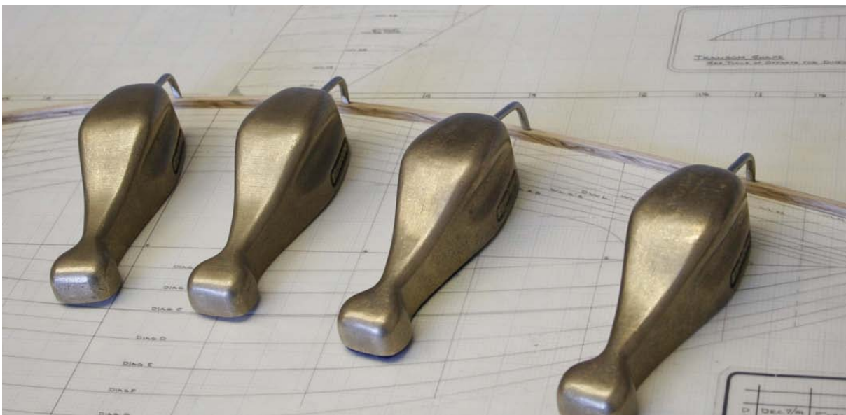
Figure 2.1: A traditional spline used for drawing smooth curves. The wooden spline is bent into shape using spline weights.
