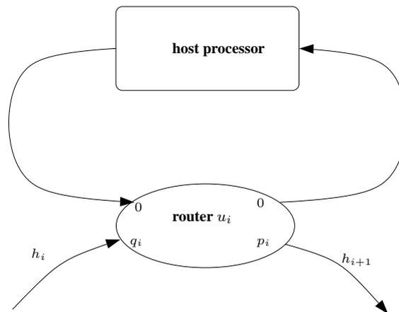
**Figure 4.1:** A model of a router
