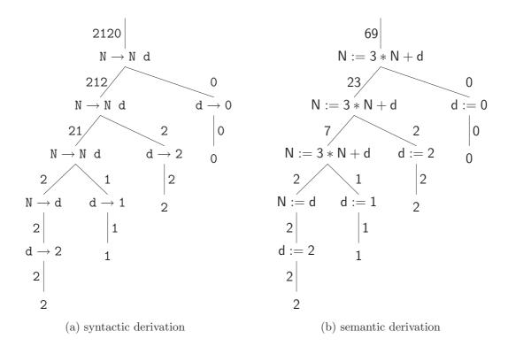
Figure 9: The analysis of a text 2120 for its numeric value  $2120_3.$
