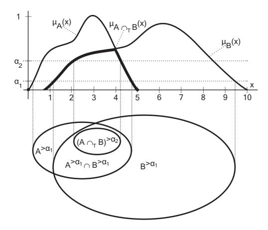
Figure 7: The alpha cut of the T-intersection of fuzzy sets.
