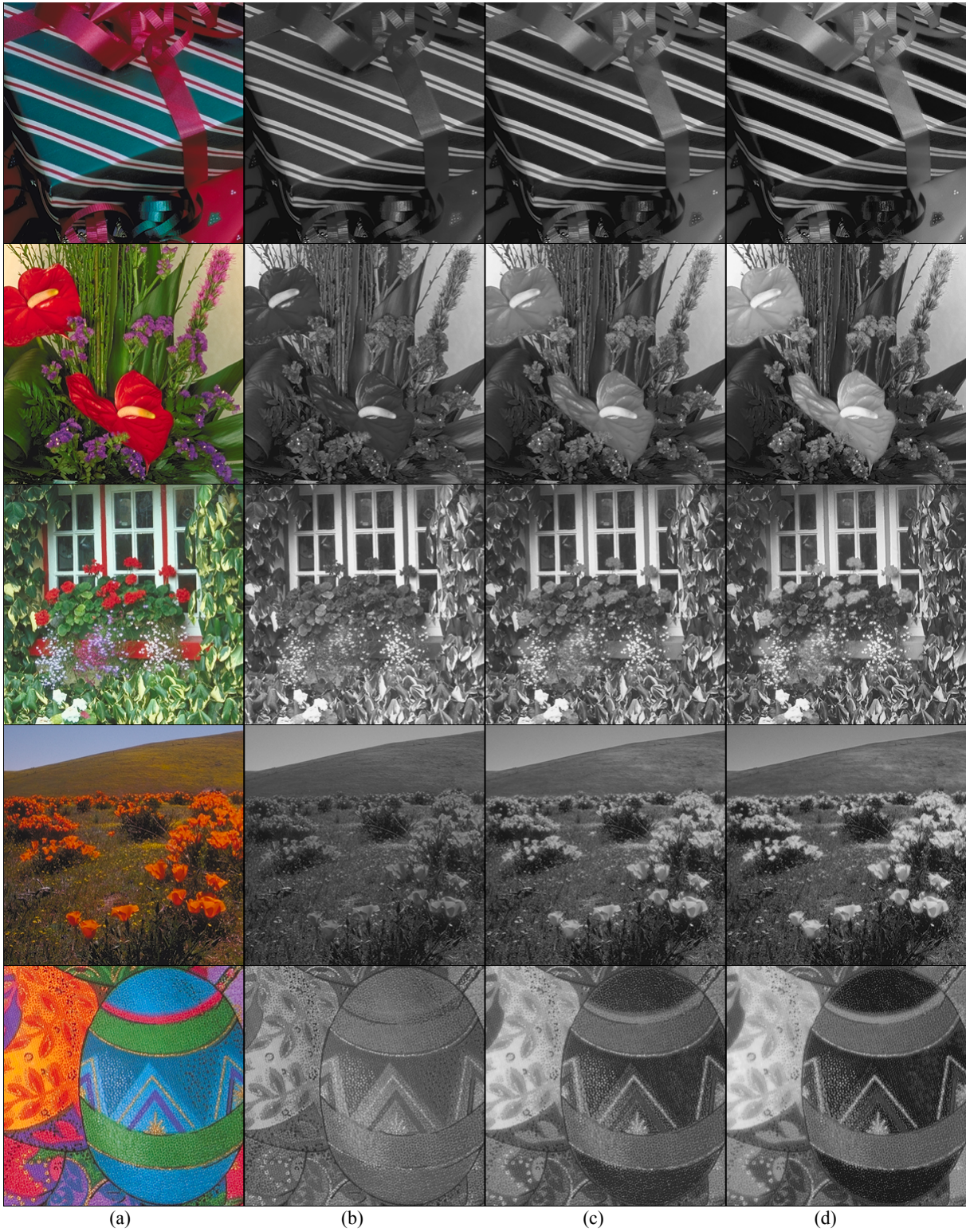
Fig. 4. Adjusting the degree of contrast enhancement: (a) color image, (b) luminance channel, (c) our enhanced grayscale with \lambda = 0.3 , (d) our enhanced grayscale with \lambda = 0.5 .
