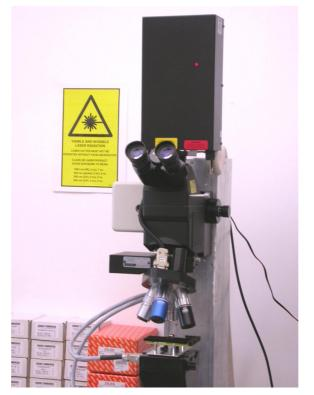
Figure 65. New Wave Research QuikLaze-II laser cutting system [128]
