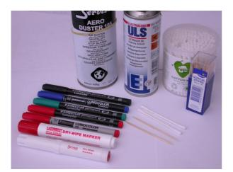
Figure 73. Tools for the toothpick UV attack
