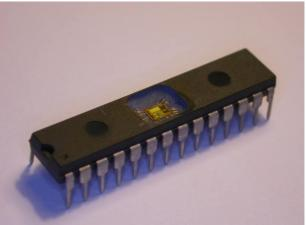
Figure 53. Decapsulated sample in DIP package
