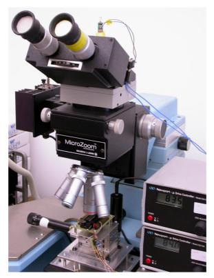
Figure 80. Laser scanning setup with the laser pointer on top of the microscope and a moving sample under it
