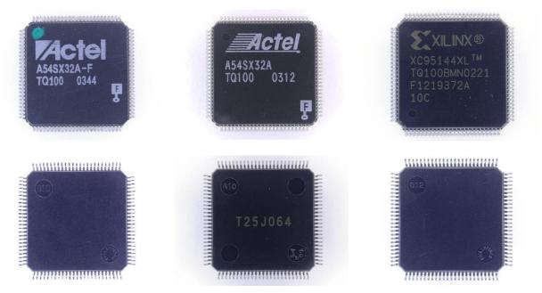
Figure 106. Remarked chip (left column) and the original Actel FPGA (middle column), and Xilinx CPLD (right column) chips from both sides
