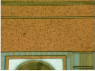
Figure 12. Second metal layer and polysilicon layer can be seen through top metal layer on Microchip PIC16F877 microcontroller [36]. 500× magnification
