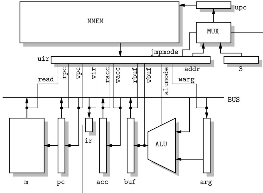
Figure 4: The AC datapath and microprogram control.
