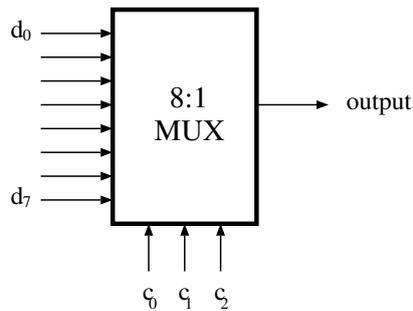
Give a circuit which implements this 8:1 multiplexer using only NAND gates. [10 marks]
