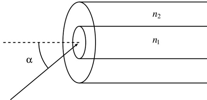
The refractive indices of the core and cladding are  $n_1$  and  $n_2$  respectively, where  $|n_1 - n_2| \ll 1$ . Prove the following condition for the incident light to be guided by the fibre
