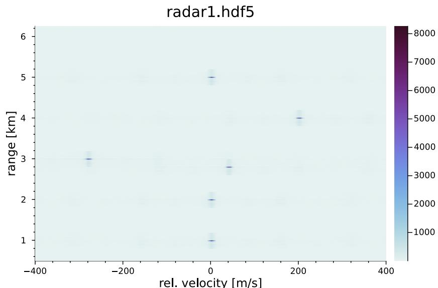
Two test recordings `radar1.hdf5` (low noise) and `radar2.hdf5` (high noise) are available on the course web pages. Each contains a contiguous complex-valued time-series vector `iq`, which represents the recorded radio signal after it was IQ downconverted from a centre frequency of  $f_c = 2.45$  GHz, then low-pass filtered with a cut-off frequency of  $B/2 = 20$  MHz, and finally sampled at a rate of  $f_s = 50$  MHz.
