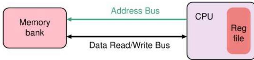
Single-core, basic computer model (no hardware concurrency).
