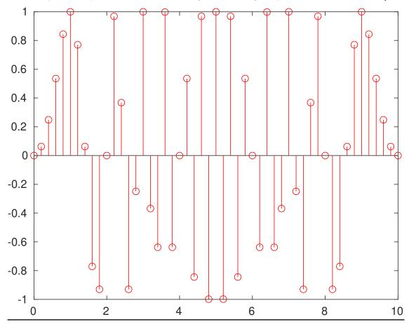
**Exercise 6:** Use MATLAB to write an audio waveform (8 kHz sampling frequency) that contains a sequence of nine tones with frequencies 659, 622, 659, 622, 659, 494, 587, 523, and 440 Hz. Append to this waveform a copy of itself in which every other sample has been multiplied by -1. Play the waveform, write it to a WAV file, and use the **spectrogram** command to plot its spectrogram with correctly labelled time and frequency axis.
