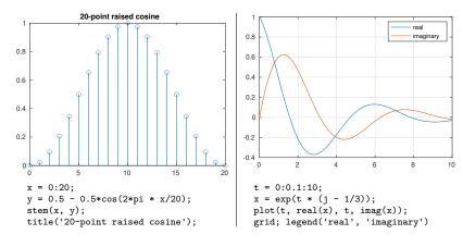
Plotting functions plot, semilogx, semilogy, loglog all expect a pair of vectors for each curve, with x and y coordinates, respectively.
