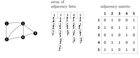
The 'adjacency matrix' representation is good if we need to be able to quickly look up for a given pair of vertices whether there is an edge between them. The 'adjacency list' representation is good if the graph is *sparse*, i.e. if there are many vertices and few edges per vertex.
