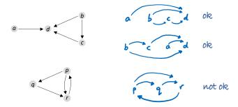
For what graphs it possible to put all the vertices into a total order? And, if it is possible, how can we compute the total order? The picture above shows two simple graphs, and three attempted total orders. The first two are valid total orders, and the third is not—and a moment's thought about the second graph tells us that it's impossible to find a total order, because of the cycle.
