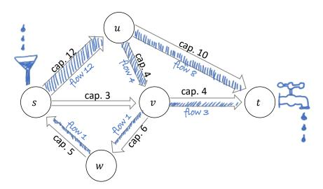
This picture illustrates a flow on a network. There are two distinguished vertices, the *source* vertex s where flow originates, and the sink vertex t where flow is consumed. The edges are directed, and labelled with their capacities. The flow value is the net flow out of the source vertex, and it's 12-1=11 in this picture. This is equal to the net flow into the sink vertex, of course.
