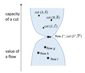
What's this theorem for? The theorem says that for any cut, every possible flow's value is  $\leq$  that cut's capacity. Likewise, for any flow, every possible cut's capacity is  $\geq$  that flow's value.
