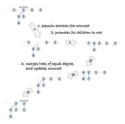
In this simple version, with only push and popmin, one can show by induction that the Fibonacci heap consists at all times of a collection of binomial trees, and that after the cleanup in lines 16–17 it is a binomial heap. (See the example sheet.)
