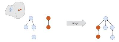
To make merge faster, we could skip all the work of updating the items in a set, and just build a deeper tree.
