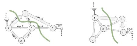
The proof is based on the idea of a *cut*. A cut is a partition of the vertices into two sets,  $V = S \cup \bar{S}$ , with  $s \in S$  and  $t \in \bar{S}$ . The *capacity* of a cut is
