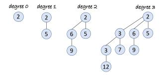
A binomial heap is a collection of binomial trees, at most one for each tree degree, each obeying the heap property i.e. each node's key is  $\leq$  those of its children. Here is a binomial heap consisting of one binomial tree of degree 0, and one of degree 3. (The dotted parts in the middle indicate 'there is no tree of degree 1 or 2'.)
