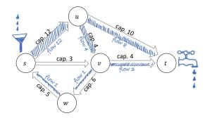
But to write a proper problem statement, we need to be more precise than this! Here are some definitions. Let the weight associated edge  $u \to v$  be  $c(u \to v)$ , and call this the *capacity* of the edge. Assume it is > 0 for every edge in the graph. A flow is a set of edge labels  $f(u \to v)$  such that
