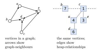
Here's a more thoughtful way to formulate the problem: When we use the Fibonacci heap as the priority queue in Dijkstra's algorithm, each vertex is doing double duty: it is at once both a vertex in the graph and also a node in the Fibonacci heap. They are participating in two data structures *simultaneously*. How should we implement this?
