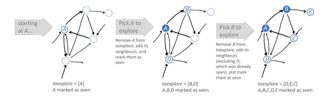
We can adapt this code to find a path between a pair of nodes: we just need to keep track of how we discovered each vertex. For every vertex at distance d, we'll store a come\_from arrow, pointing to a vertex at distance d-1. Here's a picture, then the code.
