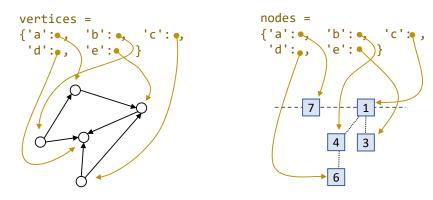
The advantage of this architecture is that it keeps the code for graph traversal entirely separate from that for the priority queue. This would be especially suitable if we start with a graph and we don't know ahead of time which algorithms we'll need to run on it; in this scenario it doesn't make sense to have a Vertex class that embodies a particular storage requirement.
