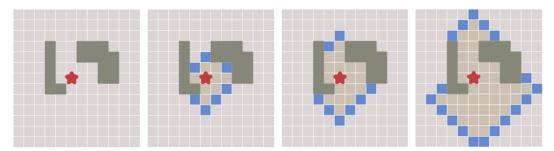
In this illustration<sup>3</sup>, we're running bfs starting from the blob in the middle. The graph has one vertex for each light grey grid cell, and edges between adjacent cells, and the black cells in the left hand panel are impassable. The next three panels show some stages in the expanding frontier.
