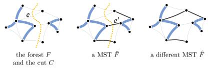
Suppose then that  $\bar{F}$  doesn't contain e. Let u and v be the vertices at either end of e, and consider the path in  $\bar{F}$  between u and v. (There must be such a path, since  $\bar{F}$  is a spanning tree, i.e. it connects all the vertices.) This path must cross the cut (since its ends are on different sides of the cut). Let e' be an edge in the path that crosses the cut. Now, let  $\hat{F}$  be like  $\bar{F}$  but with e added and e' removed.
