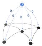
augmented graph, with an extra vertex s and zero-weight edges  $s \rightarrow v$  for all vertices v
