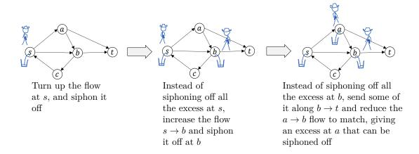
Suppose the bandits are overzealous and they discover that they can siphon off some flow at t. That means that the network operator—which was spying on the bandits all along—has learned a reconfiguration that delivers extra flow to the sink.
