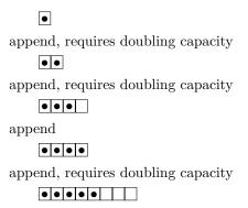
Suppose that the cost of writing in an element is 1, and the cost of doubling capacity from m to 2m and copying everything across is  $\kappa m$  for some constant  $\kappa > 0$ .
