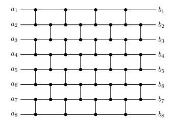
As can be seen in the figure, for i = 1, 2, ..., n and d = 1, 2, ..., n, line *i* is connected by a depth-*d* comparator to line  $j = i + (-1)^{i+d}$  if  $1 \le j \le n$ .
