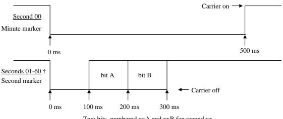
Two bits, numbered xxA and xxB for second xx bit polarity: 0=on, 1=off
