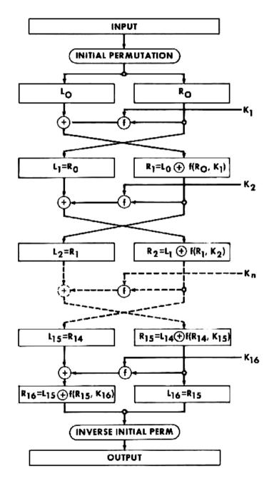
The round function f expands the 32-bit input to 48-bit, XORs this with a 48-bit subkey, and applies eight carefully designed 6-bit to 4-bit substitution tables ("s-boxes"). The expansion function E makes sure that each sbox shares one input bit with its left and one with its right neighbour.
