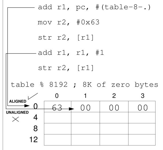
When we access words in memory the ARM expects us to provide an address where the bottom two bits are zero, this corresponds to an aligned memory access.
