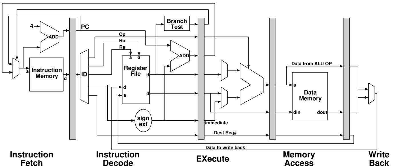
1. register bits:  $b_0$ , top bit ( $N$ ), Zero (Implement this by adding an extra bit to each register that indicates whether the current value is zero. This bit should be generated by the ALU and treated like any other register bit, i.e. all forwarding paths should be 33 bits wide)
