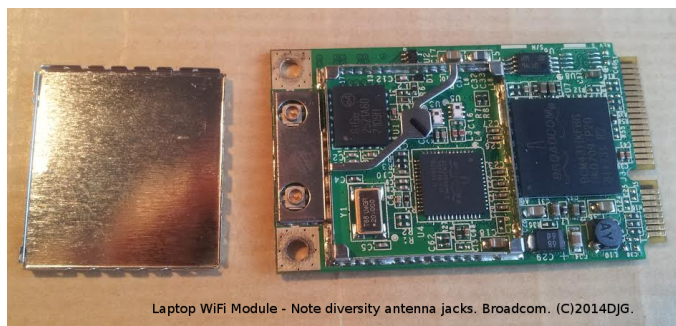
Figure 2.13: WiFi laptop module. Shielding lid, shown left, has been lifted off.
