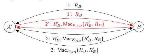
Solutions: Unidirectional keys  $K_{AB} \neq K_{BA}$  or include id of originator in MAC. Avoid using the same key for multiple purposes!
