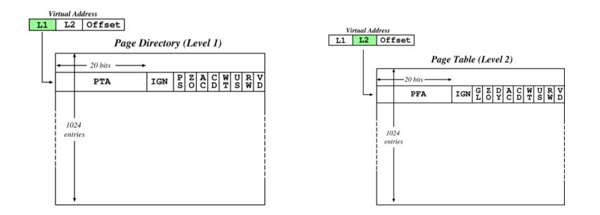
Page size is 4kB or 4MB. First lookup to the **page directory**, indexed using top 10 bits. The page directory address is stored in an internal processor register (cr3). The lookup results (usually) in the address of a page table. Next 10 bits index the **page table**, retrieving the **page frame address**. Finally, add in the low 12 bits as the **page offset**. Note that the page directory and page tables are exactly one page each themselves (not by accident)
