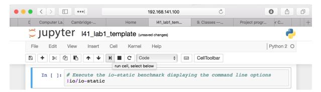
The Juypter Notebooks used for the L41 laboratories use a Python kernel running on the BBB. This allows Python scripts and Jupyter shell commands (such as those used to invoke the benchmarks) to be freely intermixed. This allows, for example, running the benchmark in a loop where each iteration uses a different set of parameters:
