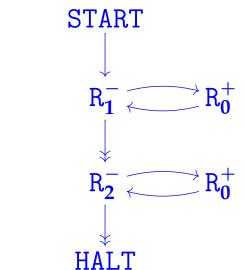
**Claim:** starting from initial configuration (0, 0, x, y), this machine's computation halts with configuration (4, x + y, 0, 0)
