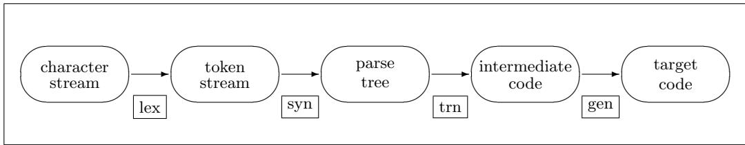
In such a compiler “intermediate code” is typically a stack-oriented abstract machine code (e.g. OCODE in the BCPL compiler or JVM for Java). Note that stages ‘lex’, ‘syn’ and ‘trn’ are in principle source language-dependent, but not target architecture-dependent whereas stage ‘gen’ is target dependent but not language dependent.
