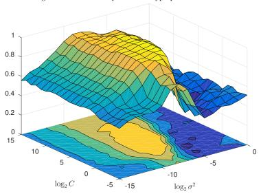
Using crossvalidation to optimize the hyperparameters C and  $\sigma^2$ .
