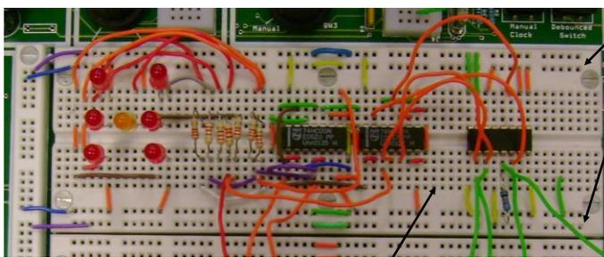
Vertical five hole strips used to connect up components
