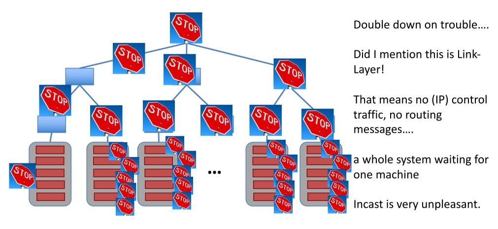
Reducing the impact of HOL in Link Layer Flow Control can be done through priority queues and *overtaking*....
