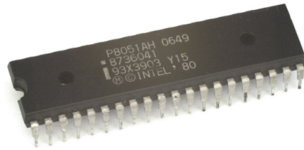
Figure 1.5: Intel 80C51 Microcontroller Chip from 1980.
