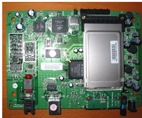
Figure 1.36: Helium chip as part of a home gateway ADSL modem (partially masked by 802.11 module).
