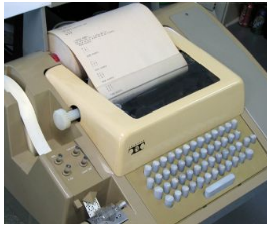
Figure 1.13: Teletype/teleprinter: These devices were almost entirely mechanical with the electric circuit being little more than one switch activated by cams for transmit and one solenoid for receive.
