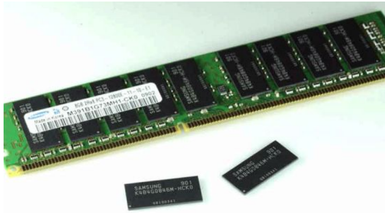
Figure 1.31: DRAM single-in-line memory module (SIMM).
