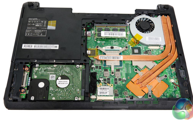
Figure 2.14: Thermal management heat pipes in a modern laptop.
