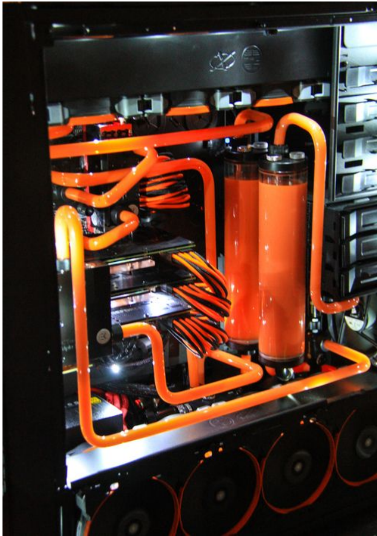
Figure 2.6: Water-cooled PC (built by Russell Hardle)
